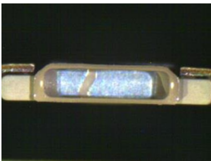
Figure 1. SMD Package After Solder Reflow Testing (aspect ratio 1:4)
